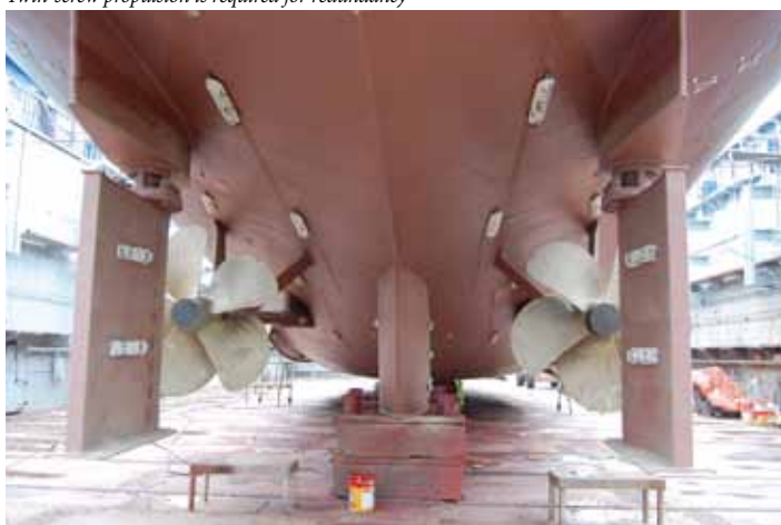
Twin-screw propulsion is required for redundancy
