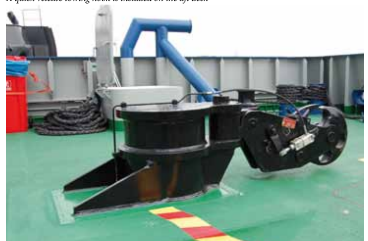
A quick-release towing hook is installed on the aft deck
